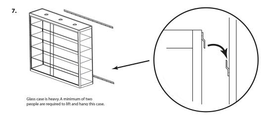
Lift case just above mounting brackets on wall. Push case to wall and slowly lower case onto brackets. Visually check that both brackets on case are seated on both mounting brackets on wall before releasing case.
